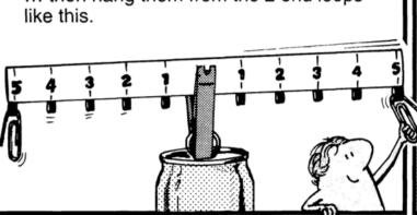
Make the beam balance level by adding a folded tape tab to the lighter (higher) side.
