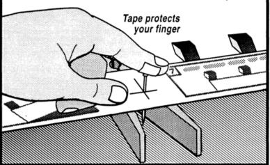
Balance your beam on the clothespin clipped on the can. The pin will rest between the "ears."
